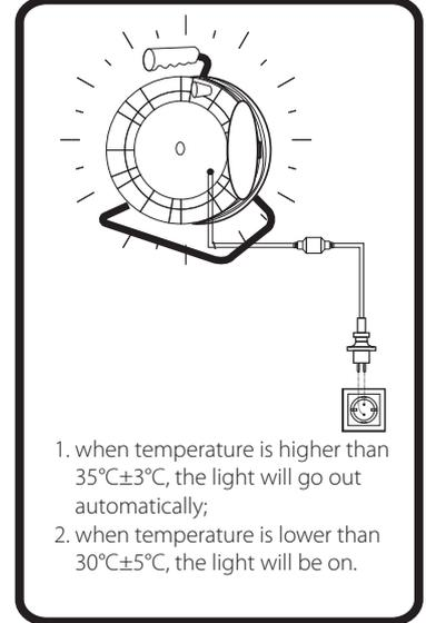
1. when temperature is higher than  $35^{\circ}\text{C}\pm 3^{\circ}\text{C}$ , the light will go out automatically;
